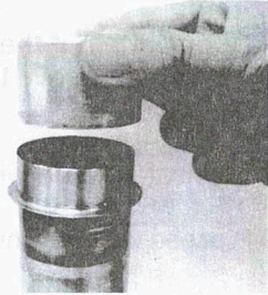
4. Put the assembly tool over the sleeve.
